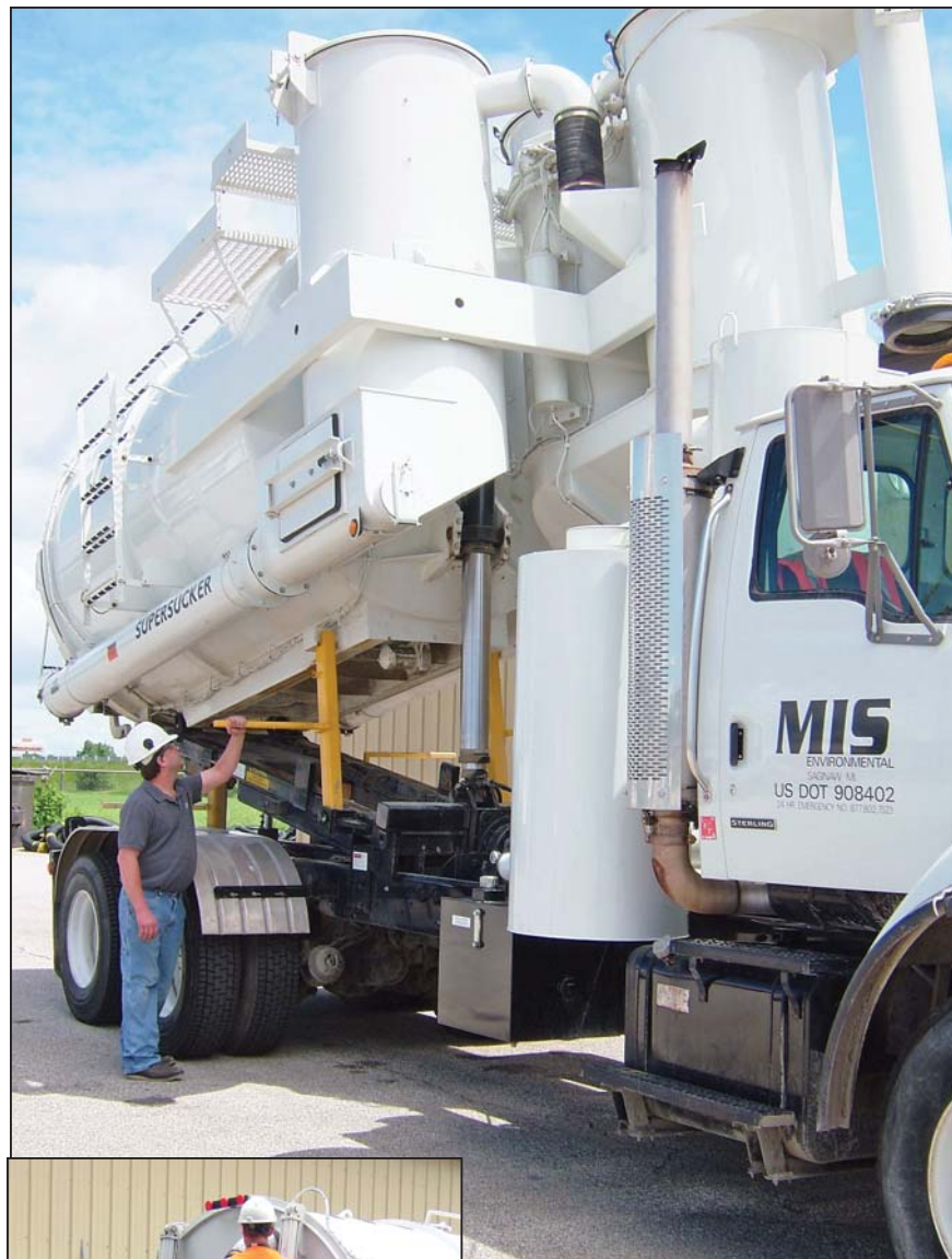
The MIS industrial vacuum fleet includes this Supersucker unit from Super Products LLC with high-dump capability.
