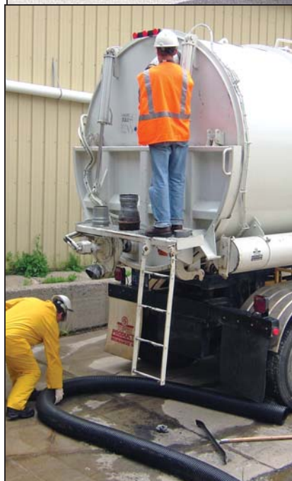
The MIS industrial vacuum fleet includes this Supersucker unit from Super Products LLC with high-dump capability.
